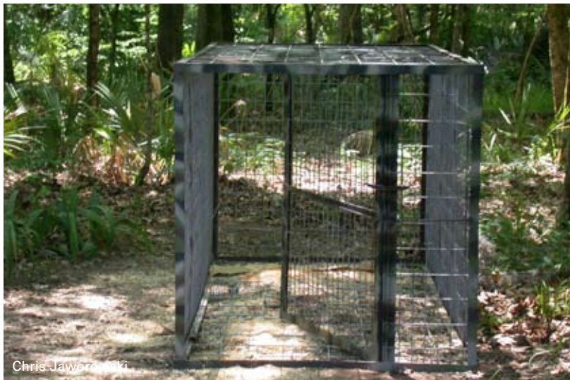
On this portable cage trap, the designer used a spring-loaded swinging door, which can be very effective.
